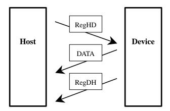
Figure 5.16 DMA data-in command protocol
